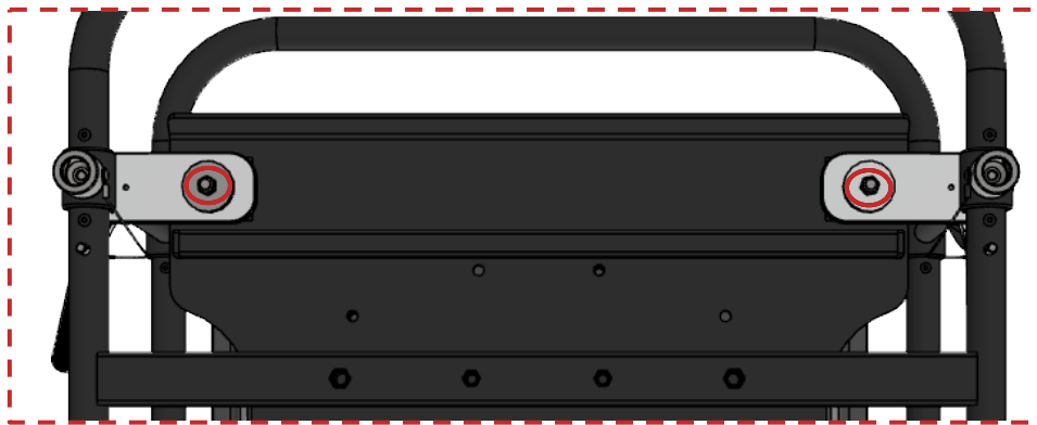
Figure 26 Nuts on front bottom side which are sealed with red colour wax
