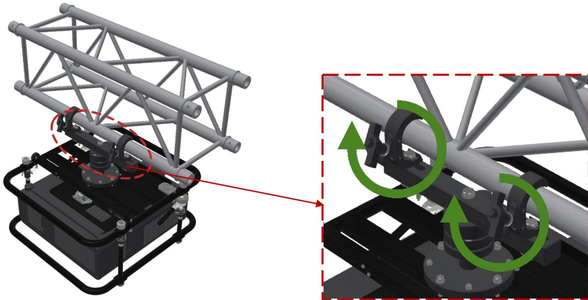
Figure 13 Tightening the wing nut on EVO-LINK-201 or -211
