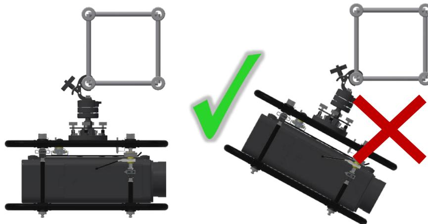
Figure 14 Only installation in vertical hanging position
