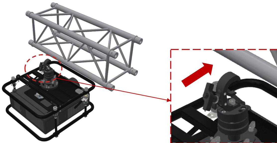
Figure 8 Mounting EVO-LINK-200 or -201 to a truss
