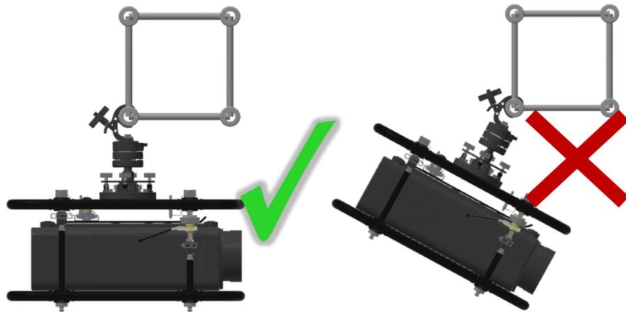
*Figure 10 Only installation in vertical hanging position*
