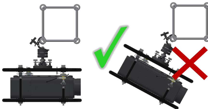
*Figure 15 Only installation in vertical hanging position*
