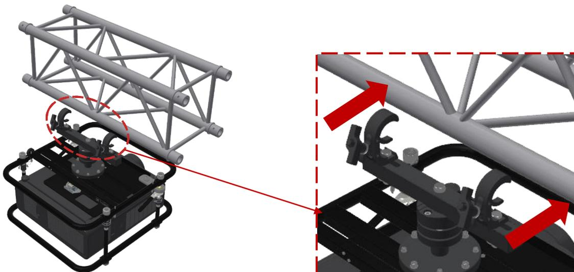
Figure 13 Mounting EVO-LINK-210 or -211 to a truss
