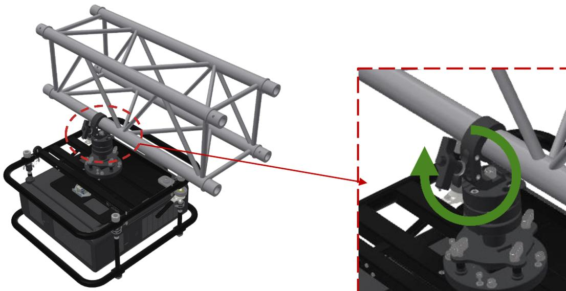
Figure 9 Tightening the wing nut on EVO-LINK-200 or -201
