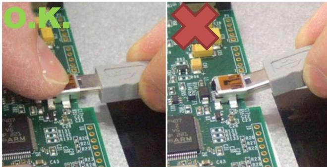
**Note:** Avoid breaking the sockets by wrong handling
