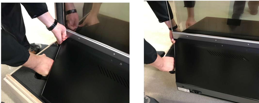
**Note:** Make sure that the GhosT-OLED cannot tilt during changing the grab of the hand on the panel unit
