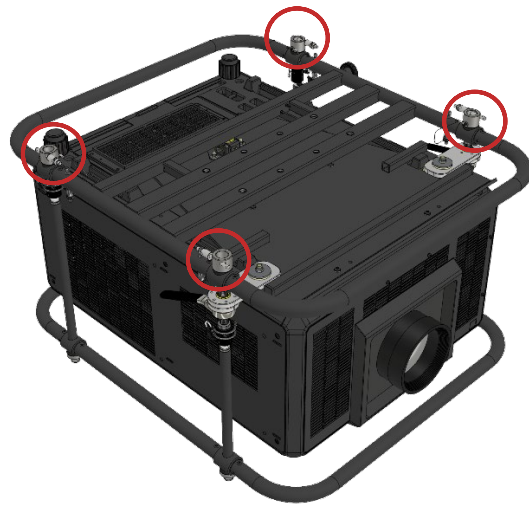
Figure 29 Stacking points bottom side
