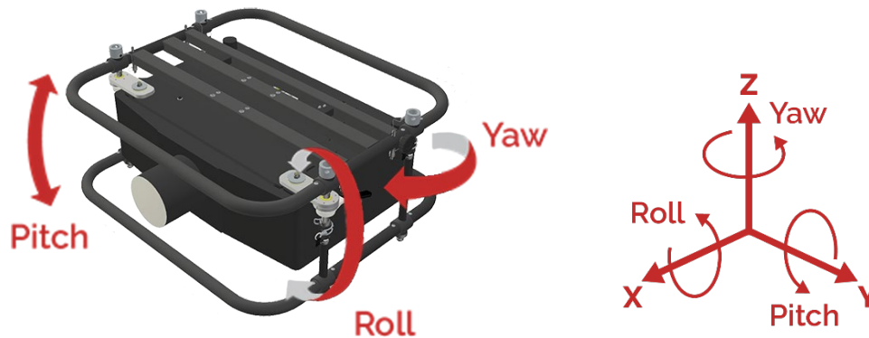
Figure 14 Illustration of yaw, pitch and roll
