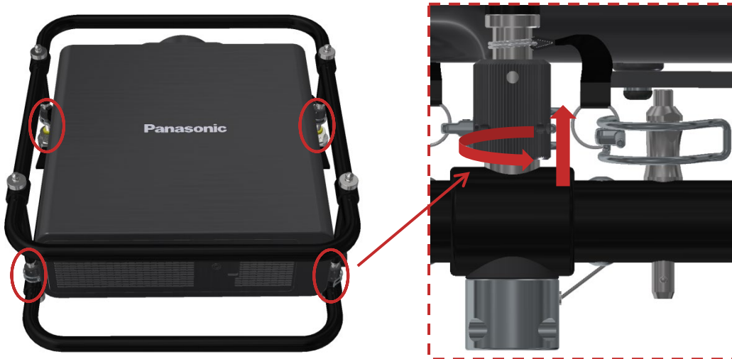
Figure 9 Unscrew the four attachment nuts
