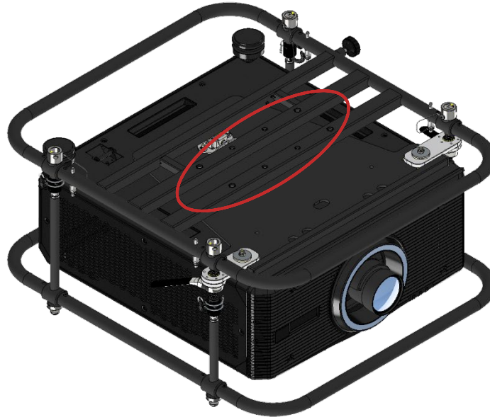
Figure 20 Threaded holes on bottom side of frame
