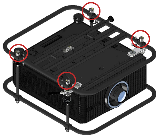
Figure 28 Stacking points bottom side
