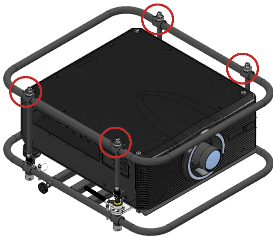
Figure 27 Stacking points topside
