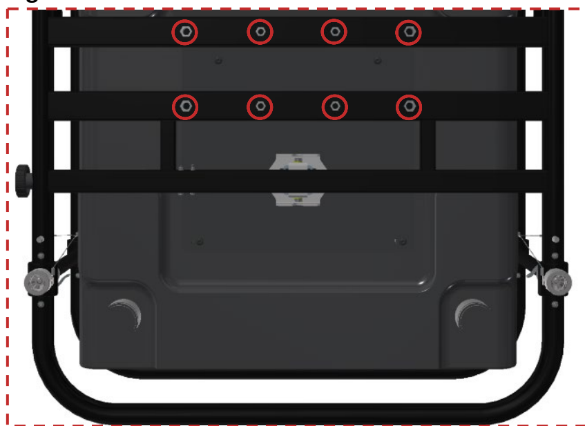
Figure 24 Inspection of mounting threads at bottom side
