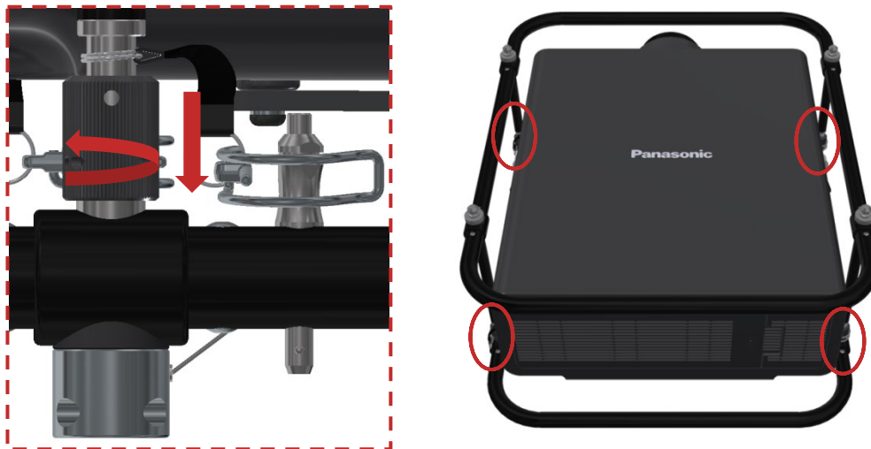
Figure 13 Tighten the four attachment nuts
