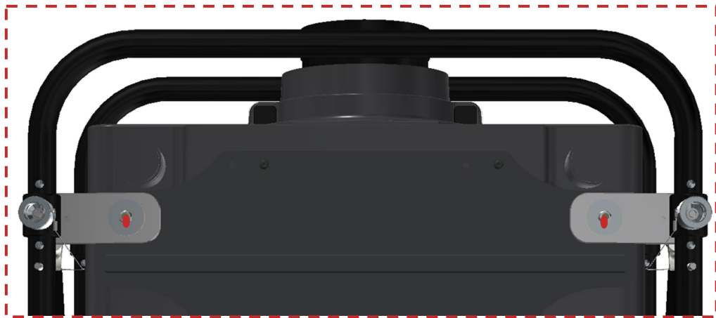
Figure 25 Nuts on front bottom side which are sealed with red colour wax
