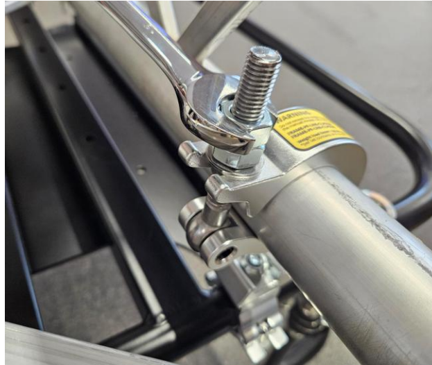
Figure 9 Tightening the second nut on the large clamp
