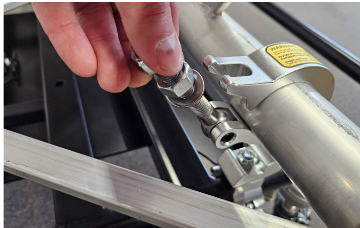
Figure 7 Mounting large clamps to supporting structure (trussing / pipe)
