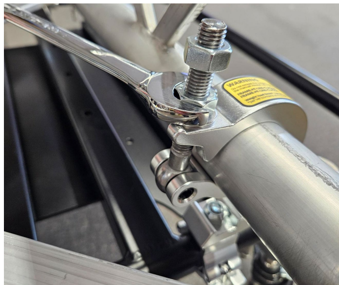
Figure 8 Tightening the first nut on the large clamp
