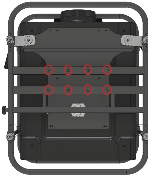
Figure 7 Bottom side of a larger frame (EVO-P20) with mounting points marked
