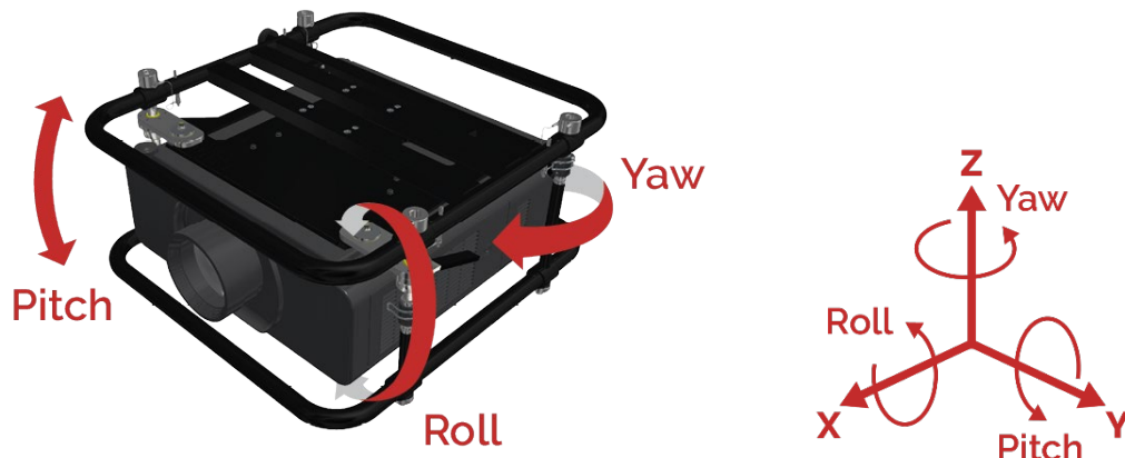
Figure 16 Illustration of yaw, pitch and roll
