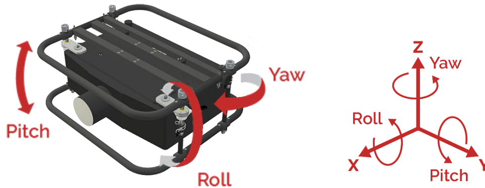
Figure 14 Illustration of yaw, pitch and roll
