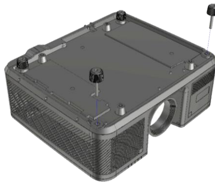
Figure 3 Remove front feet of projector
