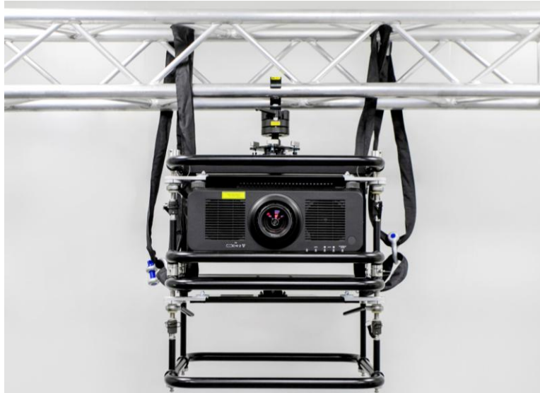
Figure 18 Securing two frames with two sets of rigging slings
