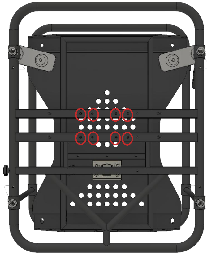
Figure 9 Bottom side of an extra large frame EVO-C40H with mounting points marked
