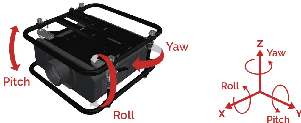
Figure 16 Illustration of yaw, pitch and roll
